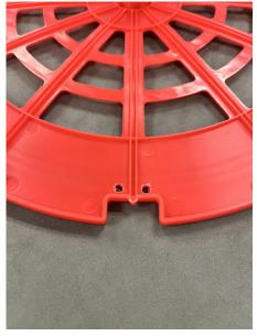
Drill two holes as pictured above. We used a 0.159" drill bit.
